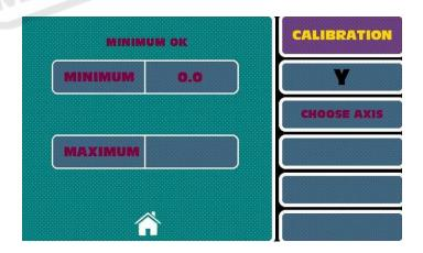
Whether an axis is on the right or left is defined by looking the machine from bracket side. Before calibrating Y axis you should set LIMIT OFF.
