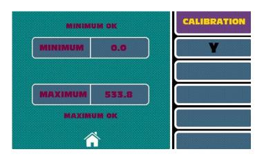
Min. Calibration is completed now. You can continue with Max. calibration.
