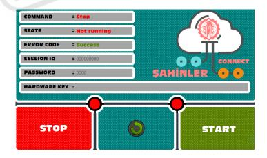
This CONNECT page is used for starting REMOTE ACCESS. If you already connected NC screen to Internet, REMOTE ACCESS can be activated by pushing START button. If connection is made successfully; you need to see this page like below:
